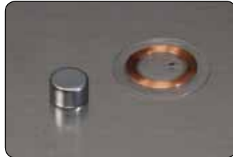
Tachometer magnet and RFID chip
